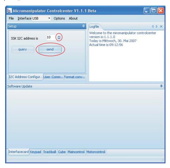
Deactivate the control and reactivate it hereon. The current address is shown on the display during the booting process.
