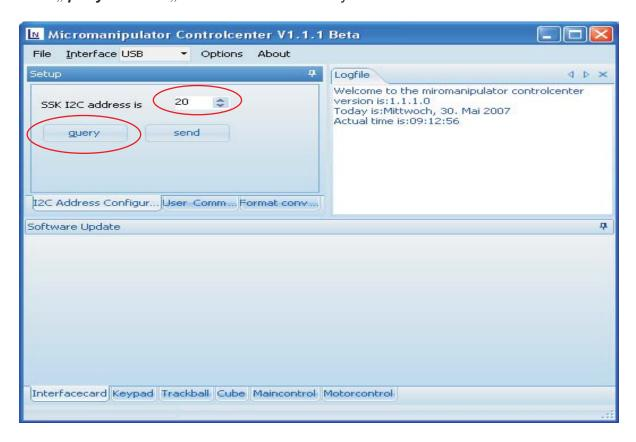
Change the address value of "SSK I2C address is" with the up / down buttons. (for master = 10, slave = 20-80) press "send"
